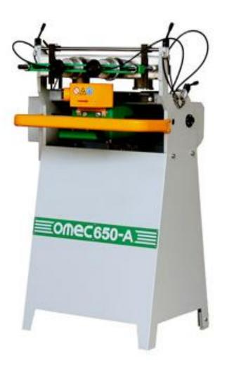
This Omec 650 is an automatic dovetailing machine. It has one milling head that cuts out all the sockets and pins in one operation.
