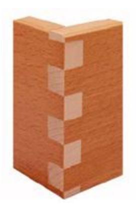
The dovetail milling head can be replaced with a straight milling head to create finger joints.
